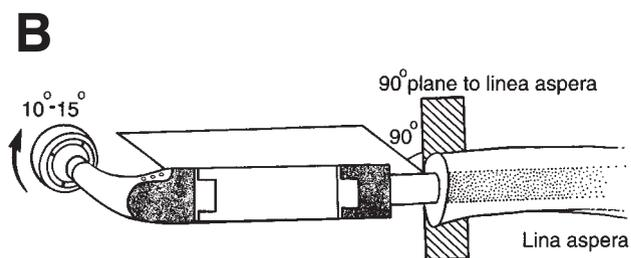
**Figure 29.19** (A) Assembly of the definitive modular prosthesis. It should match the length of the resected specimen. Note the bipolar head and the rotating hinge knee mechanism. (B) The prosthesis is positioned in  $5\text{--}10^\circ$  of anteversion with the linea aspera being the only remaining anatomic guideline for proximal femur endoprosthetic replacements and the tibial tuberosity for total femur endoprosthetic replacements.
